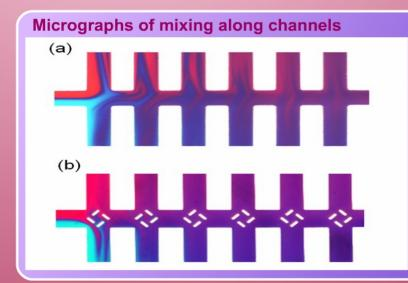
Micrographs of mixing along the unbaffled (a) / baffled (b) channel. The picture (b) indicates that more effective high frequency microfluidic mixing will be obtained by adding baffles in the main channel, which would induce the interface line to encounter more bifurcation points during high frequency oscillations.
