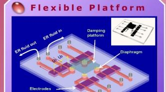
The chip sustains and controls the microplatform with four pillars. Heights of the pillars could be individually controlled by the isolated four ER fluid channels.
