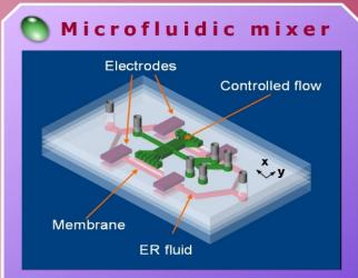
The microfluidic chip is constructed with multi-layer structure. The flow in the main channel is perturbed by liquid flow in orthogonal side channels, driven by hydrodynamic pulsating pumps, where chaotic mixing can be achieved within short passage distances.
